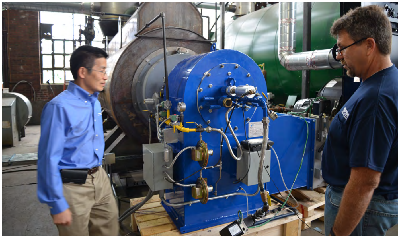
A Preferred combustion engineer and project manager work together to test the 9 ppm NO x NanoNO x burner. This production model burner was thoroughly tested in the Preferred factory to ensure a quick start-up in the field.
