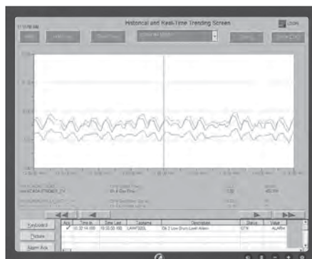
Historical Trending Display(s) An essential monitoring tool. Multiple (8) pen "Charts"
