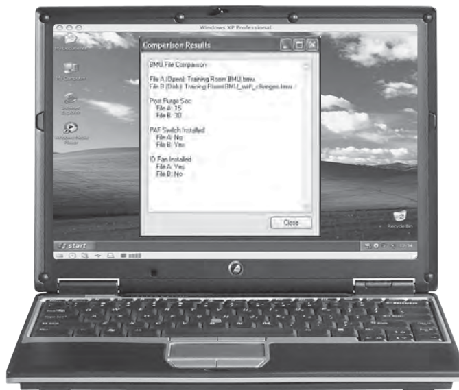
The compare function tracks any changes made to a BMU configuration for easy trouble-shooting.
