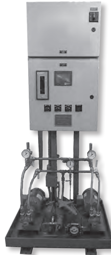
Duplex Pump Set with Inlet Oil Strainer and Pump Control Cabinet
