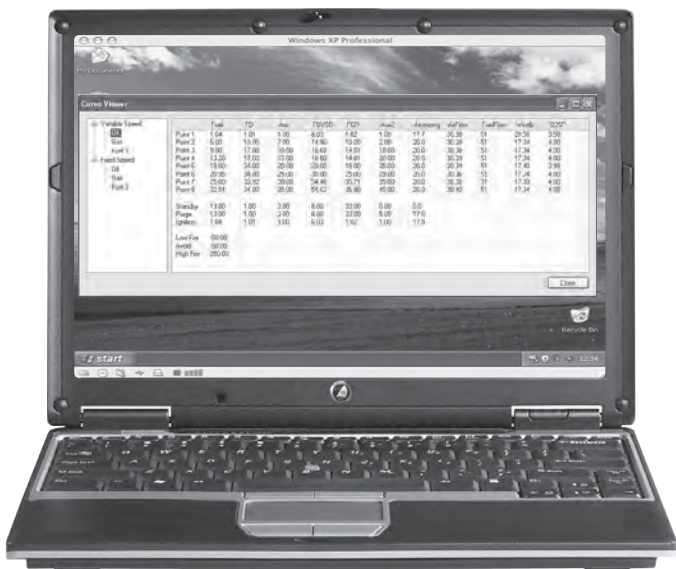
The curve viewer function allows a technician to quickly view all the combustion related curves input in a BMU. This can be useful when diagnosing a problem. It can also be used to archive curve information quickly and easily. Parameter settings and fuel-air curves can be written back to the BMU, but the points must be verified before leaving commissioning mode.
